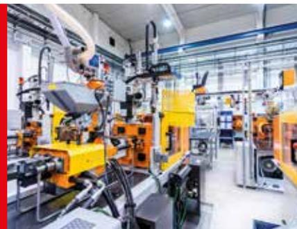
**Plastic injection moulding company Amaray produces DVD tray inlays at its production plant in Germany using two Engel Victory VC 500-150 injection-moulding machines. It needed to reduce its energy and maintenance costs and extend the machines' hydraulic-fluid-drain interval, so asked the Shell technical team for advice.**
